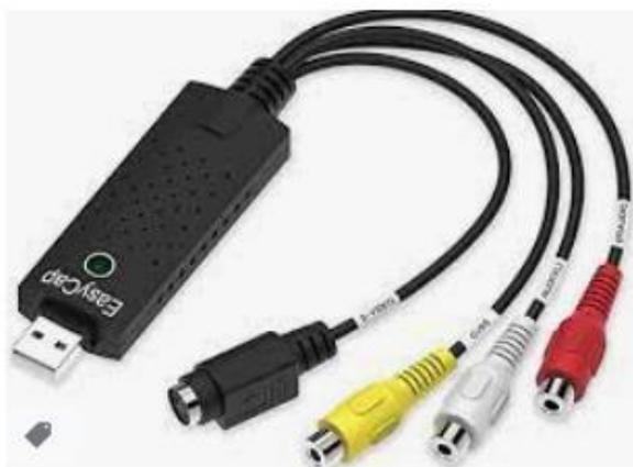
As can be seen, the main part plugs into a computer's USB port, whilst the cables connect to the VCR's "output" sockets (both video and audio).
